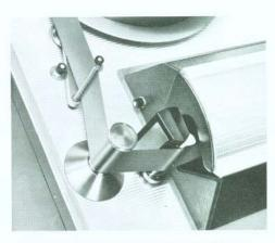
TAPE LIFTER AND CONE-SHAPED GUIDE . . . increase tape life and wear on erase head at same time reducing tape dropouts.
