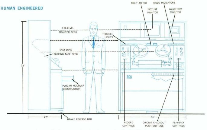
Among the human engineering features introduced in the TR-22D are a 45-degree angle tape deck set waist-high for ease in loading reels and threading tape. Recording and playback controls have been separated to minimize errors. Monitoring facilities are located at eye
