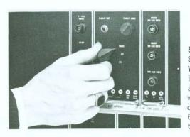
SWITCHABLE TV LINE STANDARDS FOR WORLD-WIDE USE... The TR-22D is available in a switchable standards model which provides instantaneous switchover from 525 to 625 to optional 405 or 819 tv line standards.
