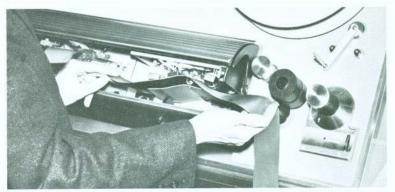
**EASY THREADING FOR QUICK-ACTION TAPE HANDLING...** Headwheel cover slides back against tape deck for easy threading... from natural, comfortable position. This expedites tape handling, splicing and editing.
